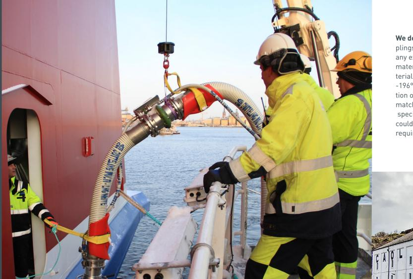
We design the widest range of DDC couplings in the world – available in almost any existing metal and many composite materials. Combined with sealing materials with working temperatures from –196°C to +280°C, and the largest variation of connections, this makes a unique match to specific requirements. To fulfil special handling procedures our couplings could be equipped to suit almost any requirements.
